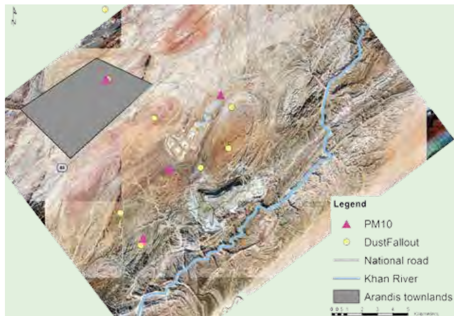
Figure 13: The map shows the PM_{10} dust monitoring network samplers and dust fall-out buckets.
